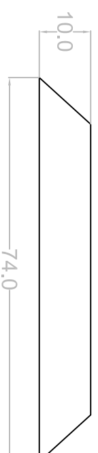
Lower cross brace (x2). 1mm thick
