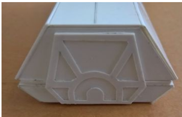
The hatch fitted to the back of the model (3mm gap to top).
